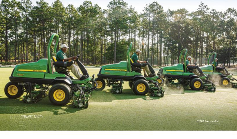
Our fairway mower lineup includes the 6080A, 6500A, and 6700A. These reasonably priced, 24.7 hp (18.2 kW) units have a lot going for them—the passcode-protected TechControl display, allowing you to control mow speed, turn speed, and more; LoadMatch™ for excellent cut quality in tough conditions; and our direct drive eHydro™ traction system, electronically controlled with no belts or linkages. Plus, all three units are built on a true fairway mower frame for toughness.
